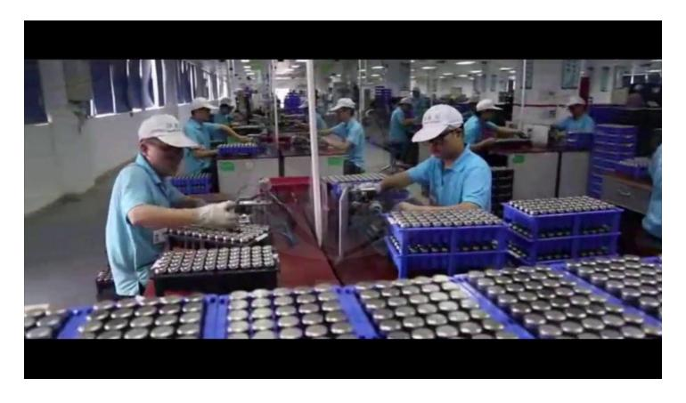
Here's how their 4680 cells are transported in racks of 8x8 cells: 64 cells each.
